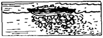
In a year's time 30 tons of barnacles can attach themselves to the bottom of an ocean-going ship.
